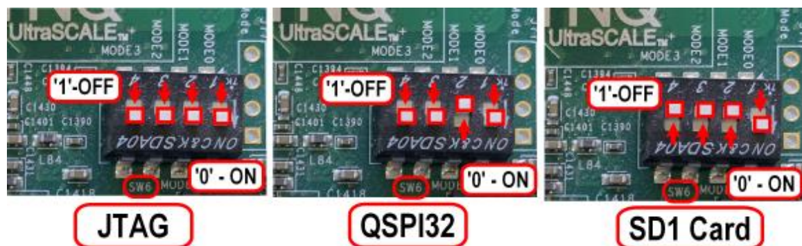
Figure 226: ZCU104 Boot Mode Switch Settings
