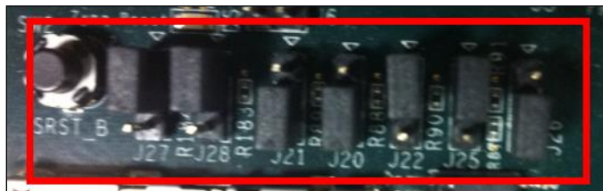
Figure 258: SD Card Boot Settings (ZC702 Board)
