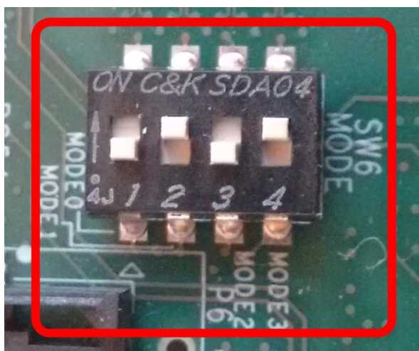
Figure 264: SD Card Boot Settings (ZCU102 Board)
